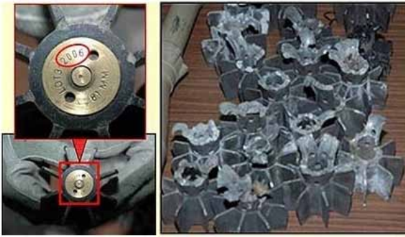
Excerpt from a U.S. government slideshow showing the remains of Iranian mortar tail-fins recovered after attacks in Iraq in late 2006. The fin configuration and design and lot number configuration identify them as Iranian munitions.
