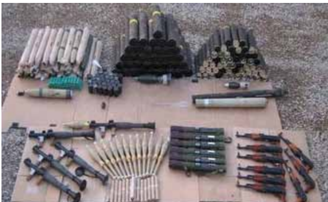
Insurgent arms cache, Baghdad 2008. Note distinctive black heat guard (used on Iranian models) in place of the RPG-7's traditional varnished-wood guard (bottom left). Also note Iranian-made 107mm rockets (top left), 81mm mortars (top right) and 120mm mortars (top center).
